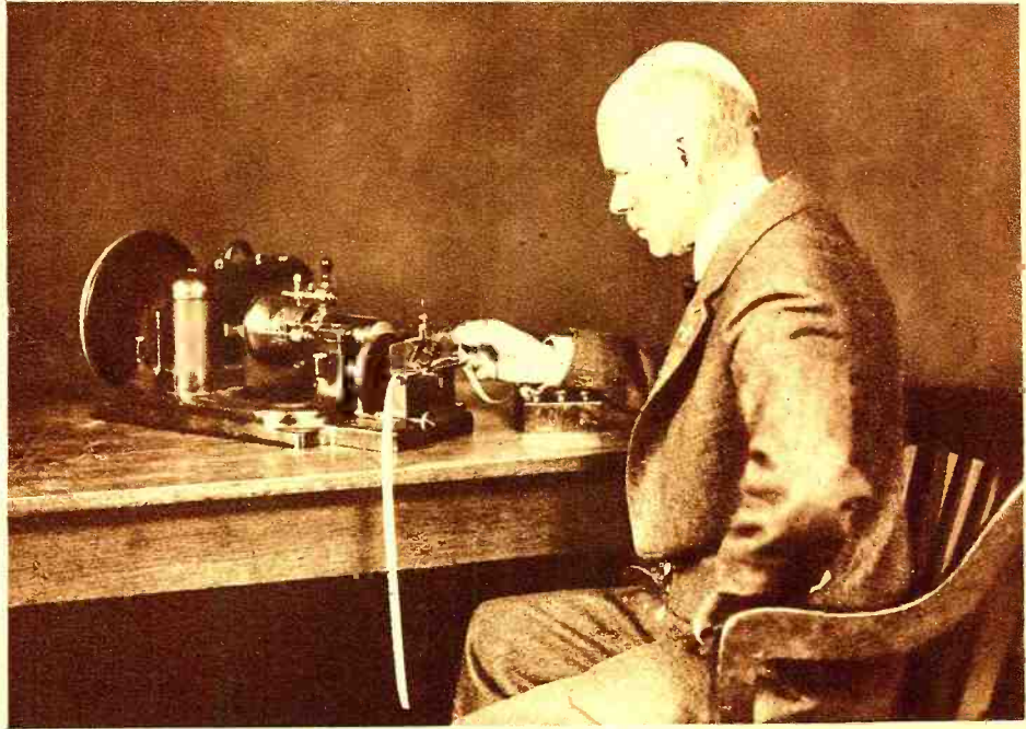
Major General George O. Squier Seated Before His Machine Which is a Portion of a New System for the Transmission of Signals at Very Low Frequencies. Instead of a Make-and-Break System the Signal Intensity is Varied.
